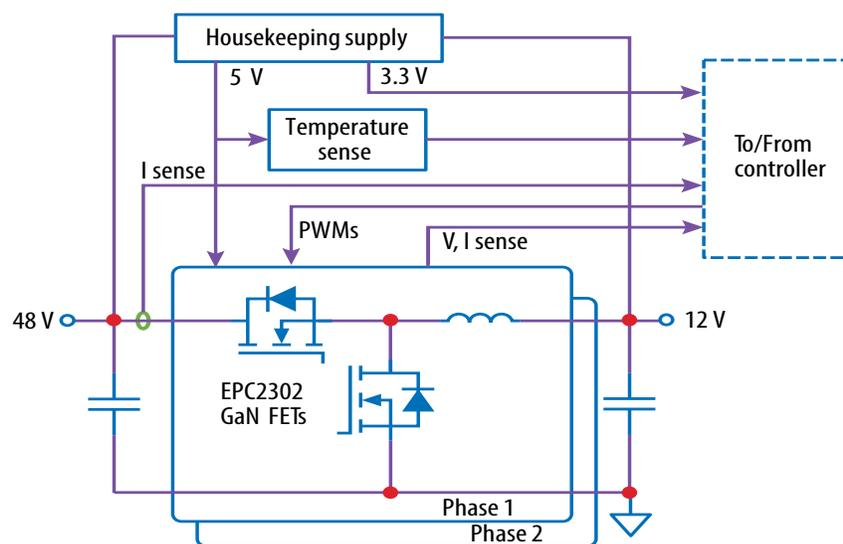
Figure 1. **EPC9165** system block diagram.
