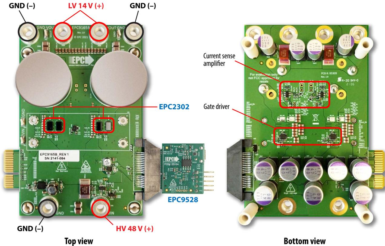
Figure 5. Photo of the EPC9165 converter with the EPC9528 dsPIC33CK controller module attached
