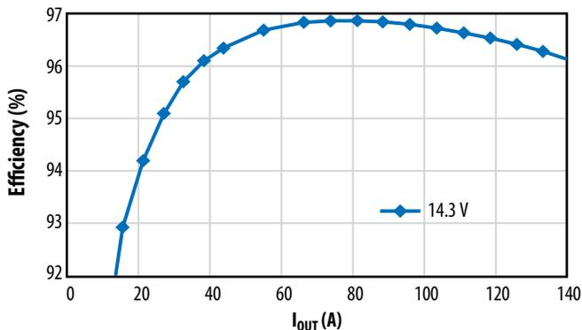
Figure 6. Measured converter efficiency at 500 kHz, 48 V input and 14.3 V output
