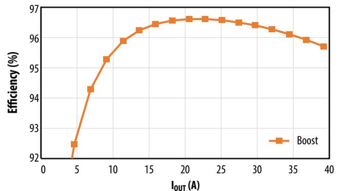
Figure 7. Measured converter efficiency at 500 kHz, 14.3 V input and 48 V output
