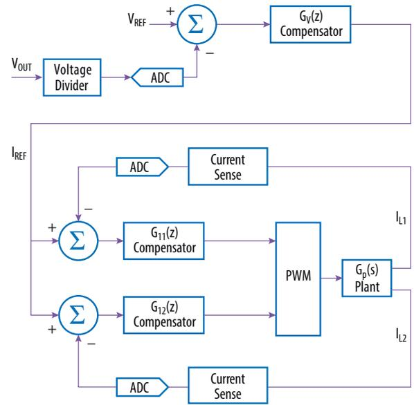
Figure 3. Digital average current mode control diagram
