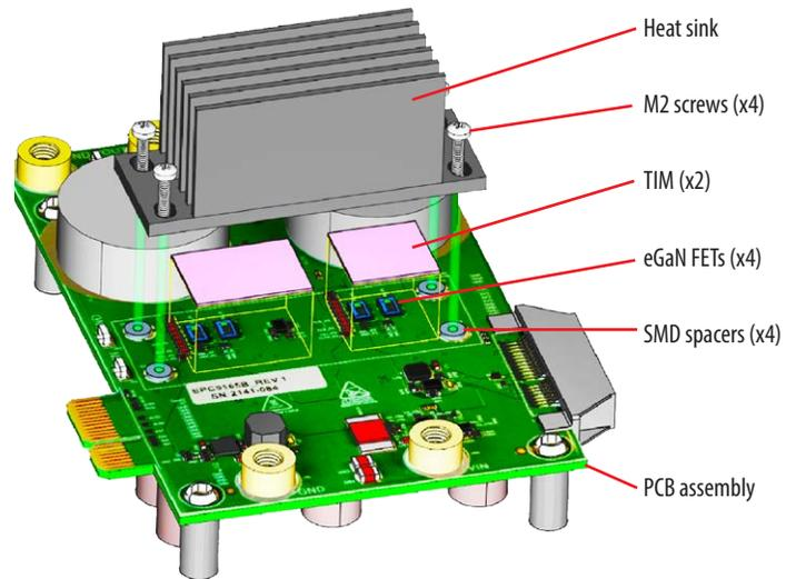
Figure 4. Heatsink installation view, showing the SMD spacers, thermal interface material
